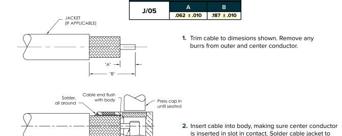
Proper assembly technique is important to the overall performance of the cable assemblies.
