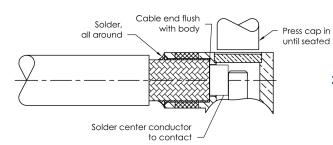
Insert cable into body, making sure center conductor is inserted in slot in contact. Solder cable jacket to body, keeping end of cable flush with step in body as shown. Solder center conductor to contact and press cap into body until fully seated.
