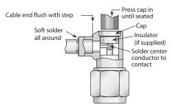
Soft solder cable jacket to body, making sure that end of cable is flush with step in body.
