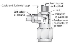
2) Soft solder cable jacket to body, making sure that end of cable is flush with step in body. Solder center conductor into contact slot, assemble insulator disc (if supplied), then press cap into body until seated or screw into place.
