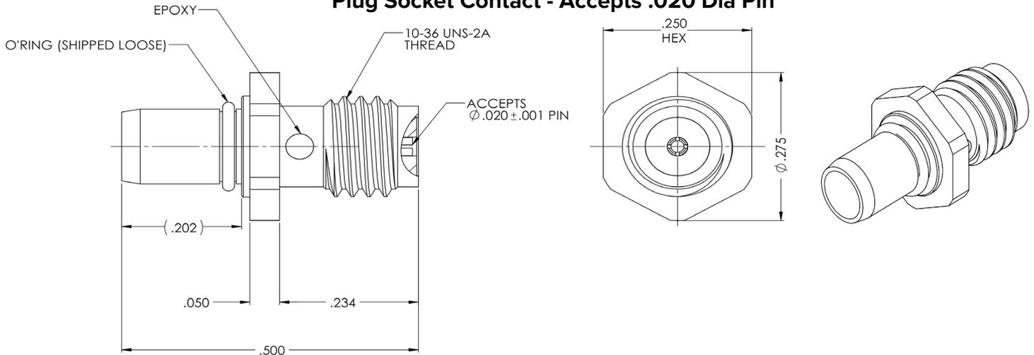
**4224025G911-000 BMMA Bulkhead Feedthrough, Cable Plug Rear Mount**
