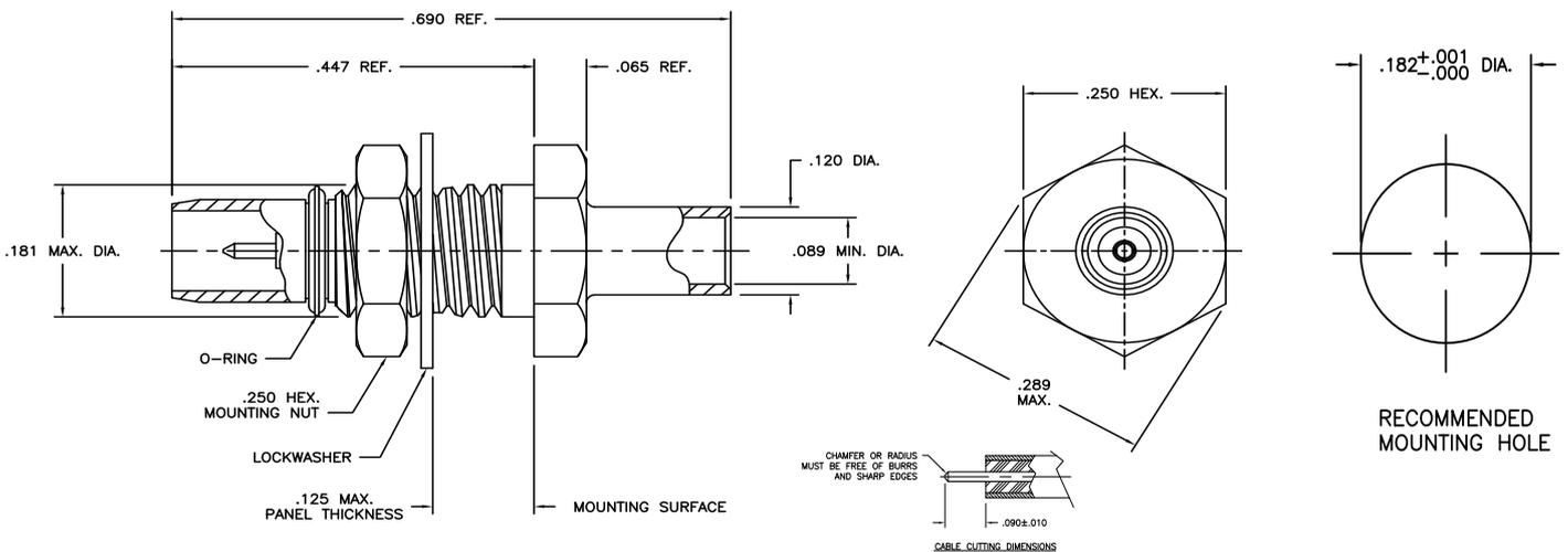
**4224000K911-005 BMMA Bulkhead Plug Receptacle - Extended Teflon & Post Contact**
