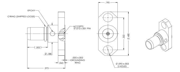
2228000K001-059 BMMA Bulkhead Jack to SMA Jack Straight Adapter
