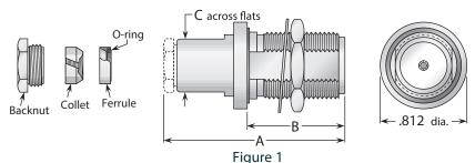
(Collet clamp [solderless] cable attachment, captive contact in body)
