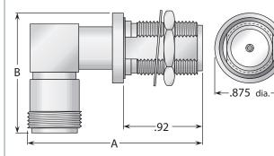
Figure 3 (Bulkhead mounted right angle jack–jack; connects two plugs)
