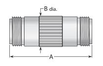
Figure 2 (Straight plug-plug; connects two jacks)
