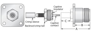
Figure 2 (Contact and insulator captive in backnut)
