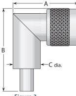
Figure 3 (Mitered body)
