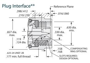
Contact Plating: Silver per ASTM B700, or Gold per MIL-DTL-45204. Gaskets: Silicone rubber per ZZ-R-765, Class II, Grade 50. Other Metal Parts: Brass per ASTM B16, plated: Silver per ASTM B700, or Nickel per AMS-QQ-N-290.
