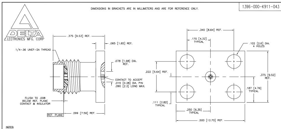
1. CONNECTOR INTERFACE IS DESIGNED IN ACCORDANCE WITH MIL-STD-348, EXCEPT AS NOTED.
